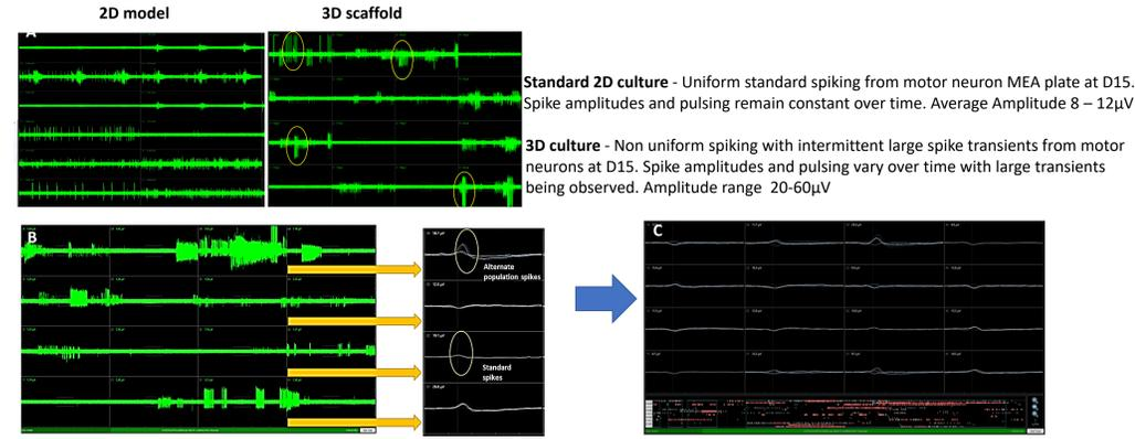
**Figure 12. Measuring 3D Network Activity.** A, Shows a comparison between a standard 2D Motor neuron network and a 3D network with a separated populations of neurons. B, comparison of the signal amplitude between 2D and 3D culture, with larger spike transients being driven by electrical input from the secondary neuron population. C, profile of synchronized firing within a well.
