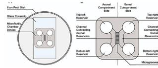
**Figure 1. Microfluidic Chamber.**
