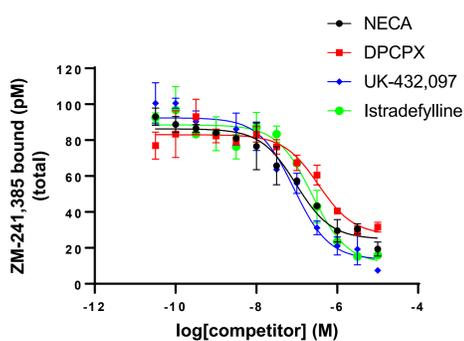
**Figure 3: ZM-241,385 as a marker ligand in competition binding studies.** ZM-241,385 at 1 nM concentration was incubated with adenosine A2A receptor membranes for 3h at 4°C in the presence of increasing concentrations of the indicated competitor ligands. Unbound ligands were removed by vacuum filtration and filter plates were extensively washed with ice-cold buffer. ZM-241,385 was then eluted and quantified by mass spectrometry. Shown is a representative graph from n=3 biological replicates.
