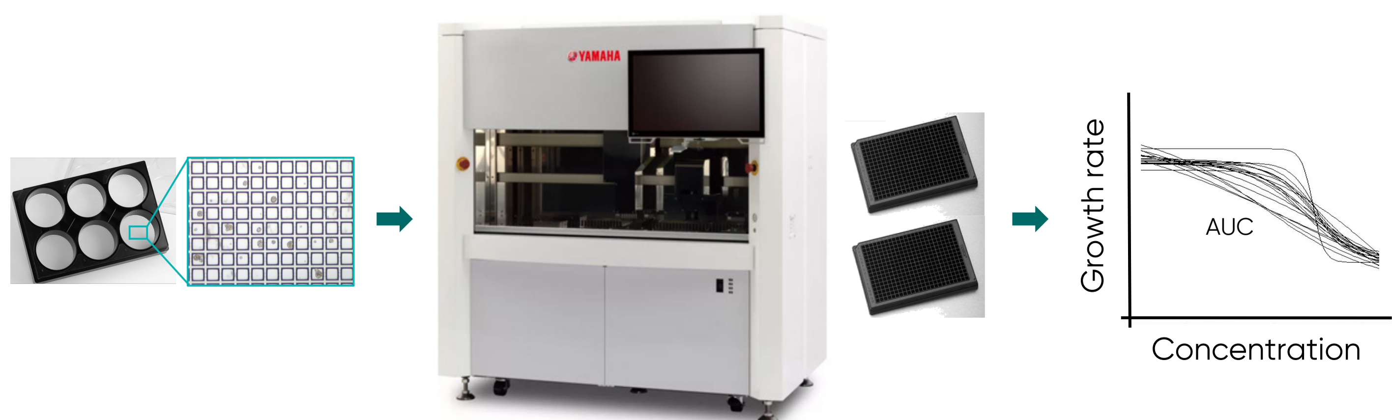
Figure 2. Yamaha CELL HANDLER: an automated system for selecting, picking and placing organoids
