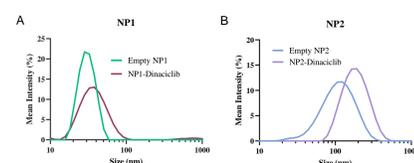
**Figure 10** Dynamic Light Scattering histograms of empty and dinaciclib loaded (A) NP1 and (B) NP2. As detailed in the table below, the hydrodynamic diameter ( $D_h$ ) of empty NP2 is approximately 3x larger than NP1 and as expected, dinaciclib-loaded particles have increased size.
